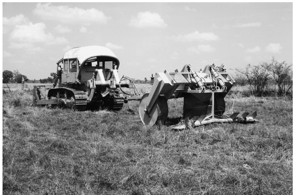
Figure 2. The blade plough and bulldozer used in this experiment.
